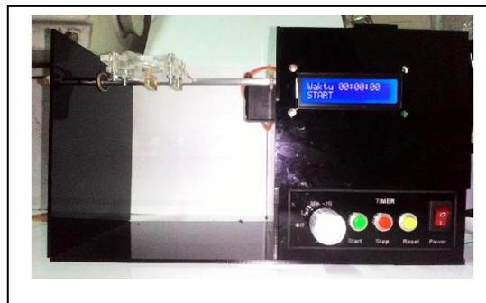
Gambar 3. Automatic chemical shaker berbasis ATmega16
