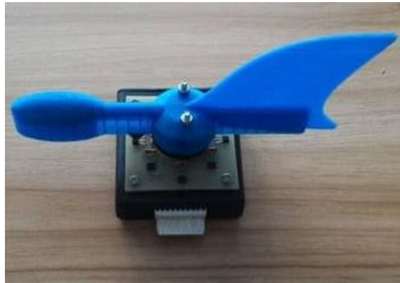
Gambar 4. Sensor Arah Angin
